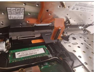
Disconnect the ribbon cable by simply lifting it up
