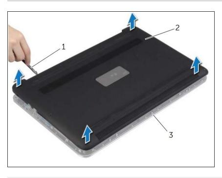
Using a spudger or some other prying tool (#1), pry off the basecover assembly from the rest of the system.
