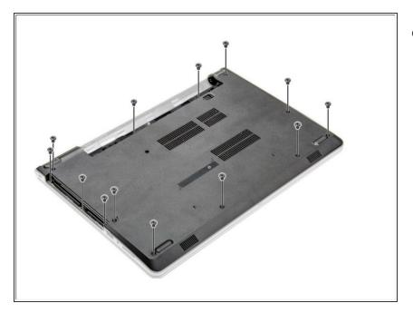
• Remove the screws that secure the base cover to the computer
