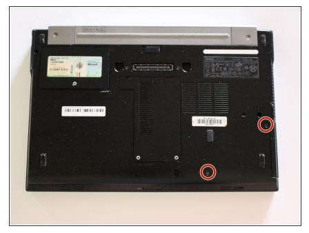
Remove the two 3mm Phillips #1 screws that secure the hard drive in place.
