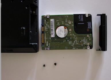
Pull the cover off of the hard drive to separate.
