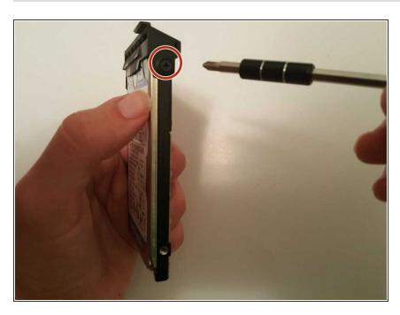
Remove the 3mm Philips #1 screw that secures the hard drive cover.
