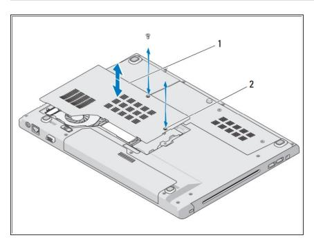
Remove the two screws that secure the memory cover, then remove the cover and set it aside.
