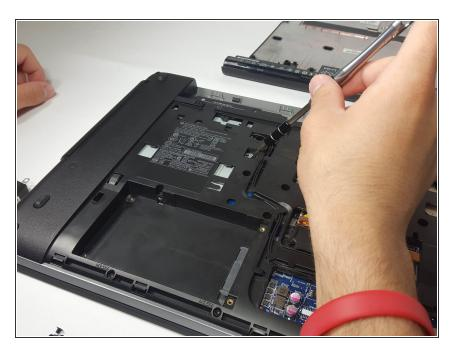
Using the screwdriver, gently push the silver tab that the screw secured to the left to release the DVD/CD drive from the computer.
