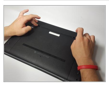
Slide the two battery release latches towards the center of the laptop to release the battery.
