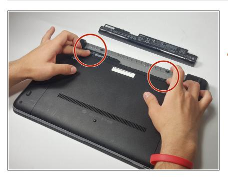
Slide the two release latches that were mentioned in the battery removal process to release the service panel.
