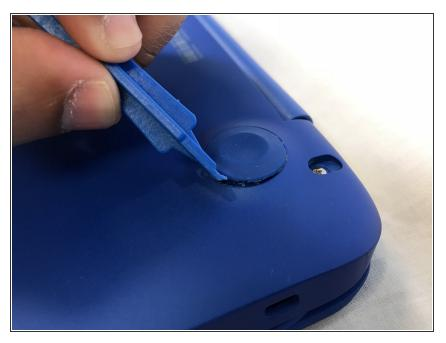
Remove the five rubber feet from the bottom of the laptop with a plastic opening tool.
