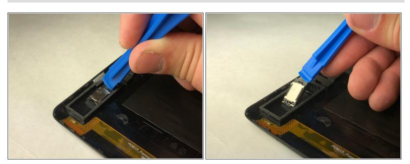
• Using the plastic opening tool, dig under the silver speaker to remove it from the back cover.
