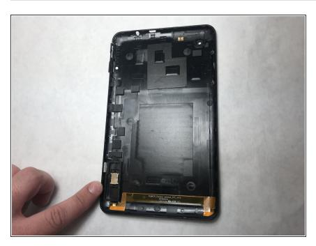
Locate the speaker on the bottom left hand side of the back cover.
