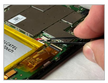
Use precision tweezers to disconnect the battery from the ZIF connector.
