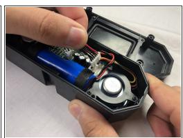
• To remove the back panel, gently pull out its wire harness.
