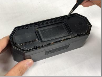
• Using tweezers, remove the four rubber stoppers in each corner of the rear panel.
