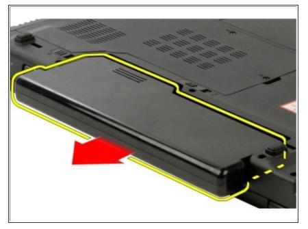
• Slide the battery itself toward the back of the computer and remove
