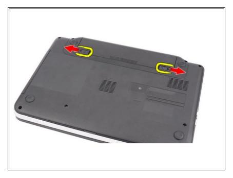
Slide the release latches to unlock the battery.
