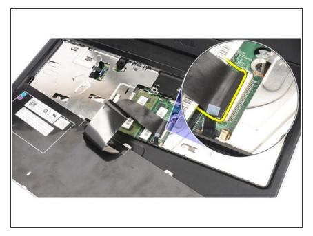
Disconnect the keyboard cable from the system board.
