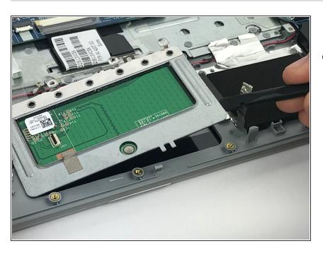
Remove the touchpad from the laptop using a spudger. To reassemble your device, follow these instructions in reverse order.
