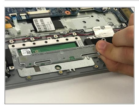
Remove the metal mounting bracket from the bottom of the touchpad
