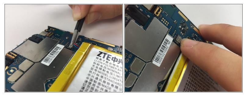
Disconnect the battery from the motherboard.
