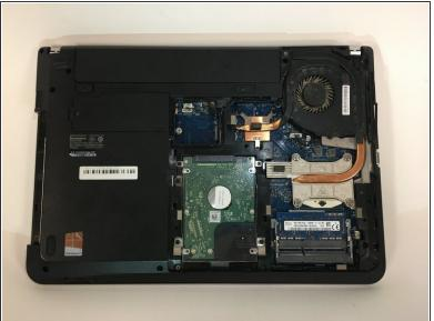
Remove the back panel of the device.
