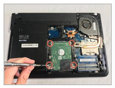
Remove four 2mm Phillips #00 screws from the hard drive.
