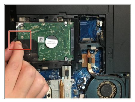
Lift the HDD upwards by pulling on the plastic tab to begin removal.
