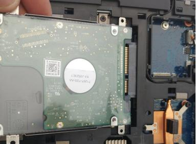
Pull the HDD out of its socket.
