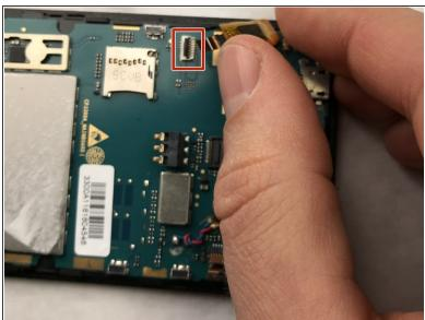
Remove the ribbon cable by flipping up the connector.
