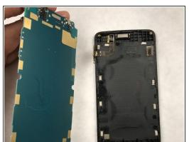
• Use the nylon spudger to gently pry/release clips to remove motherboard from the screen.
