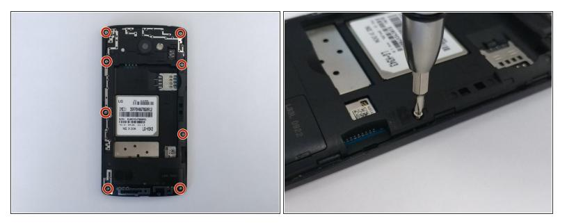
• Remove the eight Phillips #0 screws from the internal support frame.
