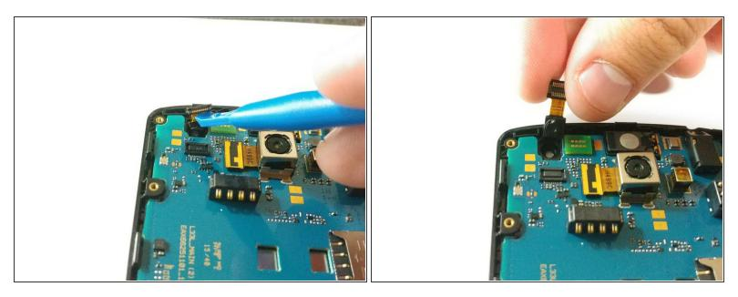
• Unclip the front camera connector from the motherboard and lift it from the frame.
