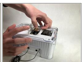
• Flip the radio over and use your fingers to lift the battery cover free.
