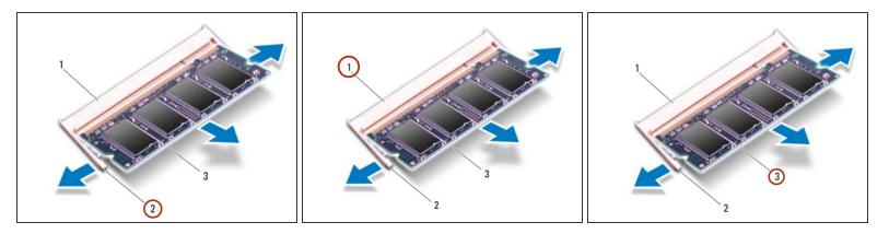
• Use your fingertips to carefully spread apart the securing clips on each end of the memory-module connector un til the memory module pops up.
