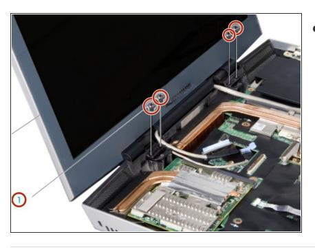
Replace the four screws (two on each hinge) that secure the display assembly to the computer base.
