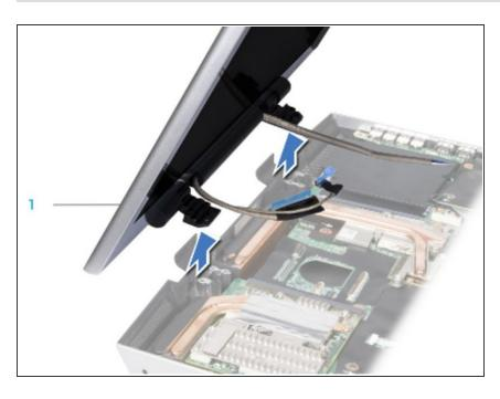
Bend the display assembly towards the computer base at a 45-degree angle and lift the display assembly off the computer.
