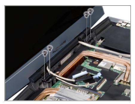
Align the screw holes on the display hinges with the computer base.
