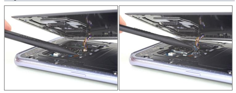
• Use the point of a spudger to pry up and disconnect the fingerprint sensor flex cable.
