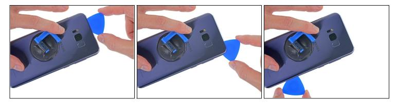
• Slice through the remaining adhesive along the top edge and right side.
