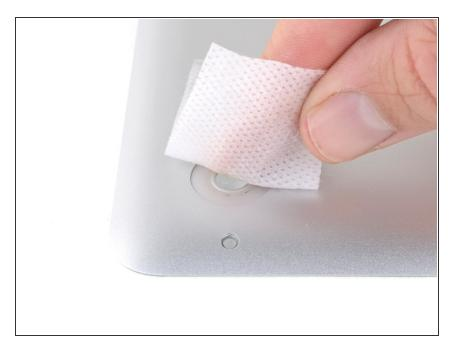
Wipe the foot pad with an alcohol prep pad to remove any residue left by the cleaner.
