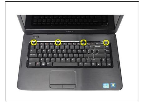
Pry up to release the tabs securing the keyboard to the computer.
