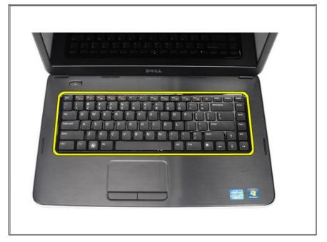
Flip the keyboard and lay it on the palm-rest.
