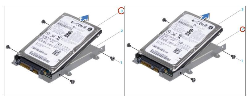
Slide the hard drive out of the hard drive bracket.
