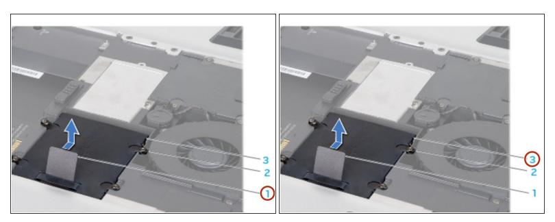
Using the pull tab, slide the primary hard drive (HDD0) towards the back of the hard drive bay and lift it out.
