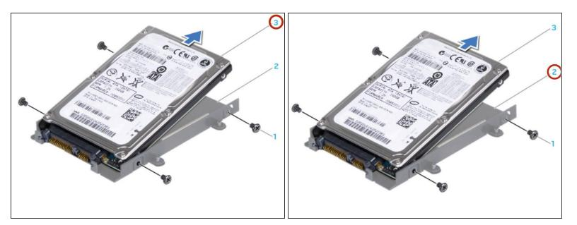
Slide the hard drive into the hard drive bracket.
