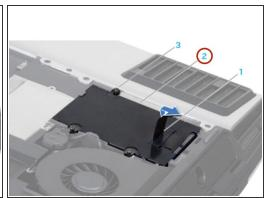
• If your computer has a secondary hard drive (HDD1): **1.** Loosen the four captive screws on the secondary hard drive (HDD1). **2.** Using the pull tab, lift the secondary hard drive (HDD1) out of the hard drive bay.
