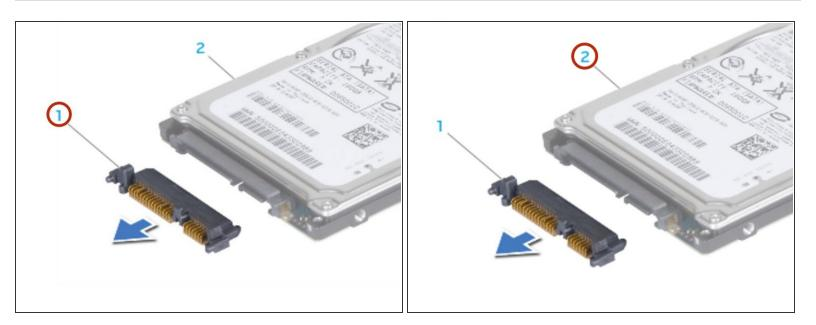
Remove the interposer from the secondary hard drive (HDD1), if applicable.
