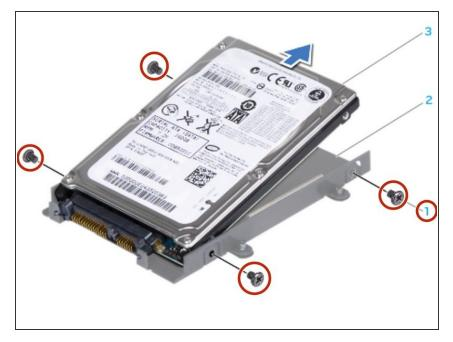
Remove the four screws that secure the hard drive bracket to the hard drive.
