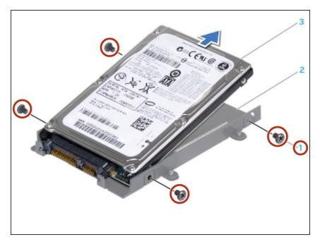
Replace the four screws that secure the hard drive bracket to the hard drive.
