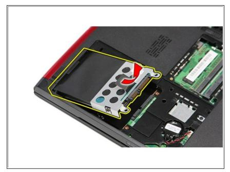
Pull up on the black hard-drive release tab and lift the hard-drive assembly up and away from the computer.
