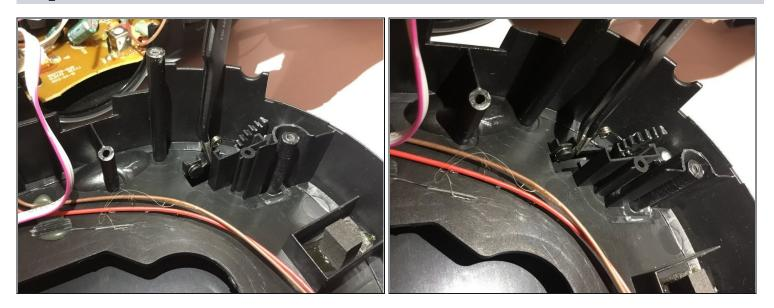
• Grasp and remove the spring using tweezers.
