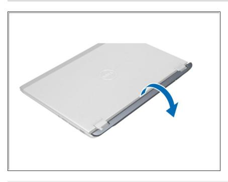
Remove the display-hinge cover from the computer.
