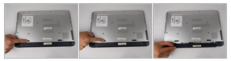
• Slide the battery release switch to the right until the battery pops out.
