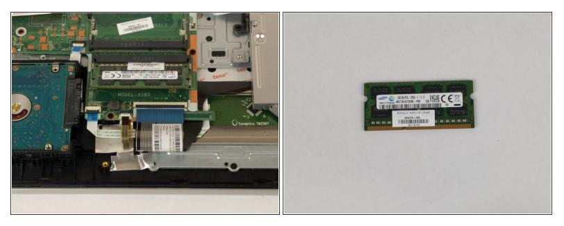
The card will pop up when silver retainers are released. The card is ready to remove, pull straight out.
