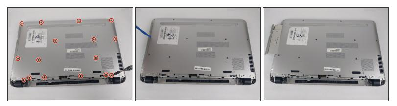
Remove all 16 of the 3.5 mm screws with a PH1 screwdriver and pry/slide the CD drive out of laptop.
