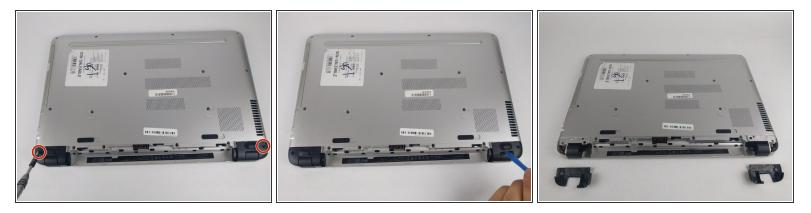
With the battery removed, remove both black plastic covers with a plastic opening tool. Unscrew both 7.5 mm screws from the tabs, using a PH1 screw driver. Using a plastic opening tool, pry off both covers.
