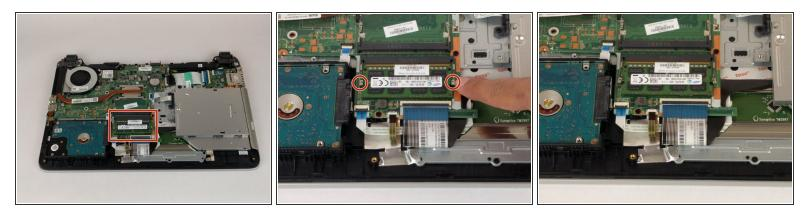
• Locate the RAM stick, will be next to hard drive. Unclip the two silver retainers on each side.
