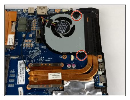
Use a #0 Phillips head screwdriver to remove the two 7mm screws holding the fan to the motherboard.
