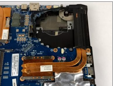
Lift the CPU fan out and replace with the replacement fan.
