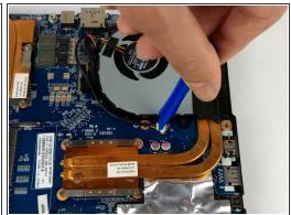
To take out the CPU fan it is necessary to disconnect the CPU fan cable. Use a plastic opening tool to remove the cable.
