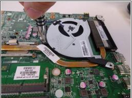
Use the PH1 Screwdriver to remove the two screws (7 mm) which hold the fan in place.
