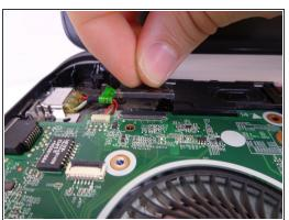
Remove the display connection wire. Lift the connection straight up from the motherboard.
