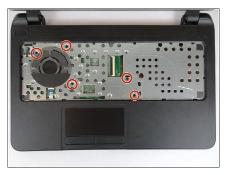
Remove the five 7mm Phillips #1 screws found underneath the keyboard.
