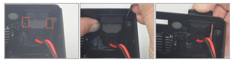
Using the small plastic splunger, press in on the two latches on the sides of the power supply switch, then push it out of the case.
