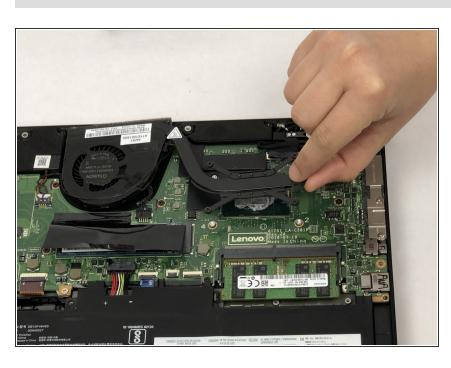
Using your index finger and thumb, gently pry the cooler from its mountings and remove the assembly. To reassemble your device, follow these instructions in reverse order.
