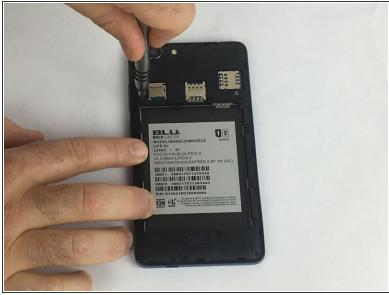
Remove twelve 2.1mm Phillips #000 screws from the rear plate.
