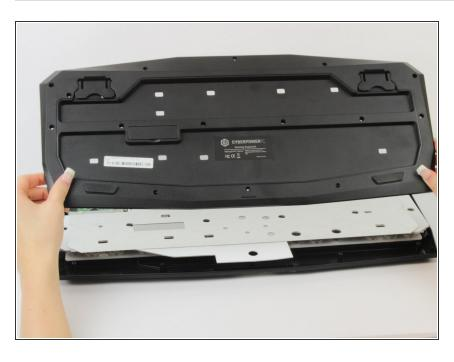
Lift up and remove the plastic casing.
