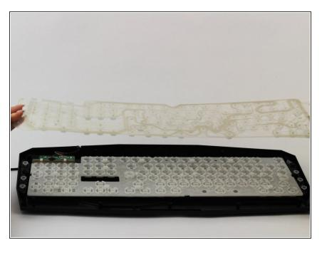
Now the cell membrane should be exposed, gently lift this part and ensure that the rubber buffers are all
