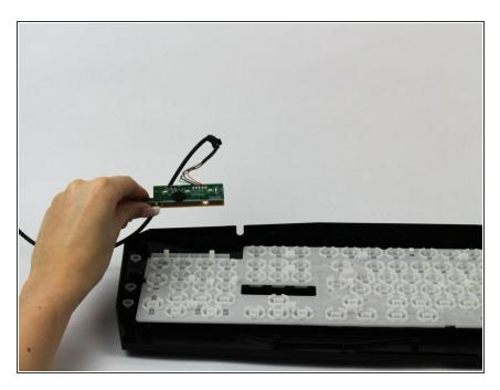
Remove the motherboard and its attached cable from the plastic casing. The cord should now come free to replace.
