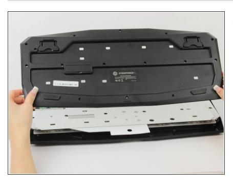
Lift up and remove the plastic casing.
