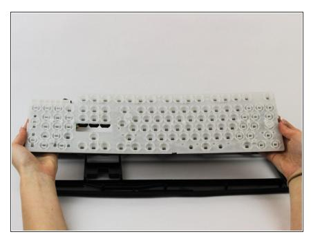
The keyboard should now be free to move, pick up the entire keyboard membrane and search for the key that needs to be replaced, to assist in remembering which key needs to be replaced place a small marker dot on the individual key back.
