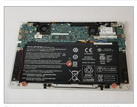
Unscrew the marked 1.5 mm screws with a Phillips #01 screwdriver.
