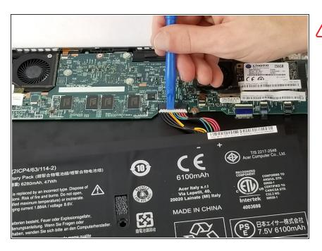
Disconnect the cable located at the top of the battery. Be careful to pull the cable horizontally, not vertically.
