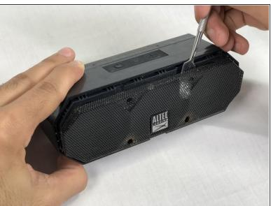
Pry off the wire mesh on both sides using a metal spudger.
