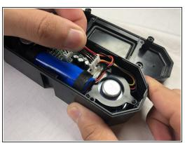
To remove the back panel, gently pull out its wire harness.
