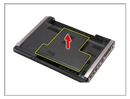
Lift up the base cover and remove it from the computer.
