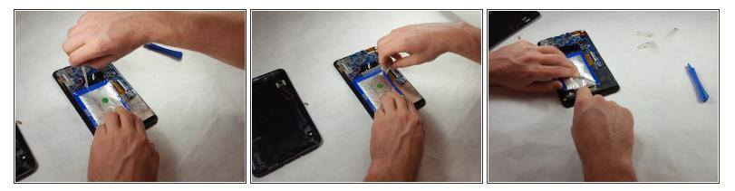
• Remove the three pieces of adhesive placed over the edges of the battery.
