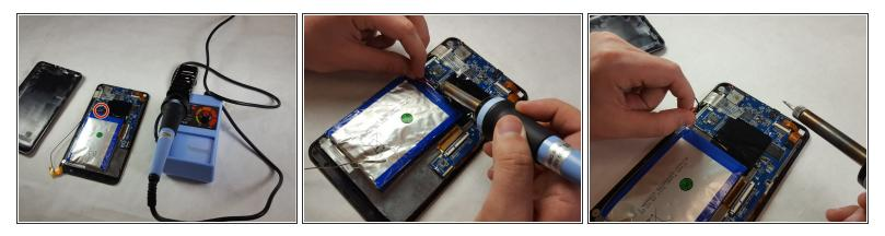
• Heat up the soldering iron, proceed to desolder and remove the battery connections.
