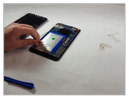
• Remove the wifi antenna from the bottom of the battery.
