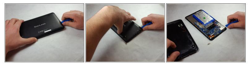
• Remove the device's back cover using the plastic opening tool.
