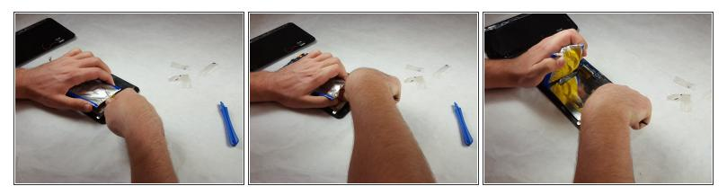
• Remove the battery from the casing using a nylon spudger.
