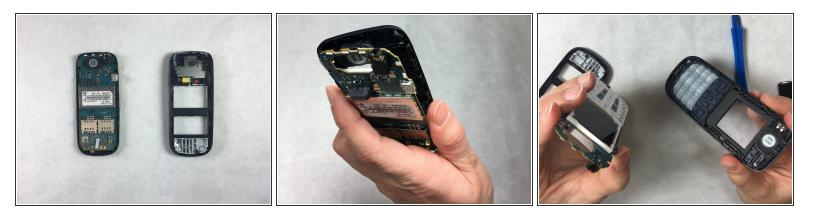
After separating the front and back components of the phone, proceed to take off the motherboard. This can be done by releasing the plastic clamps on the corners and edges of the plastic front using your fingernail.
