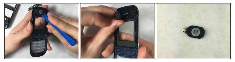
• Lastly remove the speaker using the plastic opening tool.
