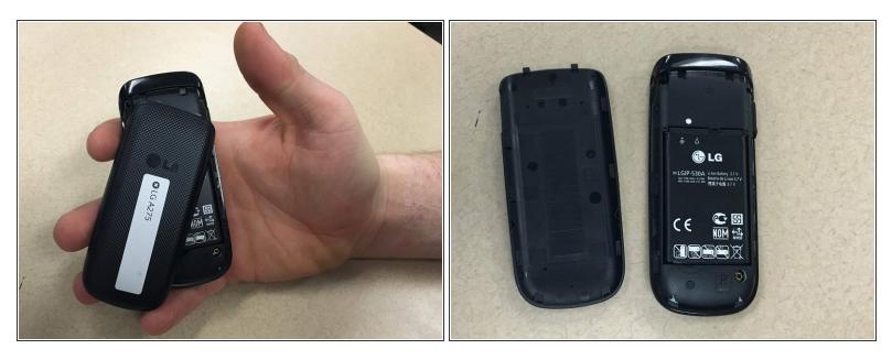
Slide the back down towards you and remove the back cover. You should hear a slight click as the cover comes off.
