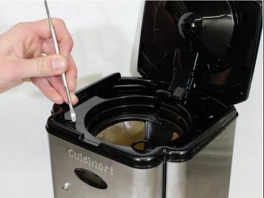
Using the metal spudger, gently pry out the two plastic plugs located on top.
