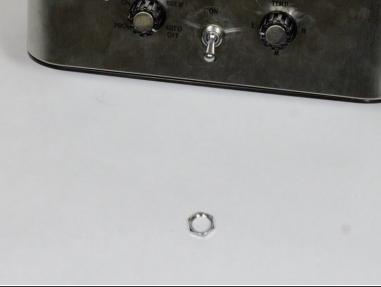
Remove the hex nut from behind the toggle switch on the front of the face plate.
