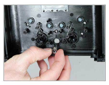
Remove toggle switch by pulling it out from inside the face plate.
