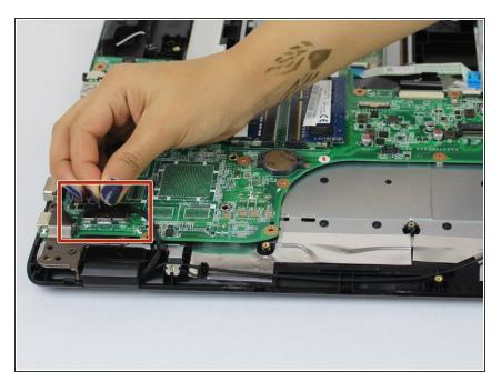
• Disconnect the display cable from the motherboard.
