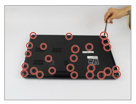
Remove the twenty-five 6mm Phillips #0 screws from the bottom panel of the laptop.
