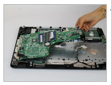
Lift the motherboard up from the narrow side and jiggle slightly so that way it doesn't get caught on the ports of the laptop case.
