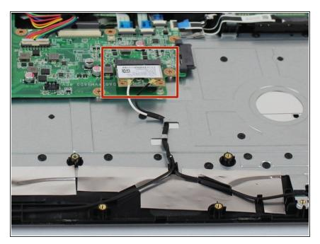
• Remove the Wi-Fi card by pulling it from the motherboard socket.
