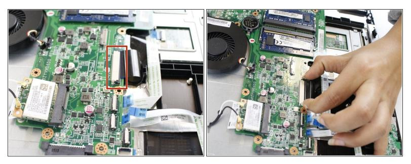
Use a spudger to flip up the retaining flap on the black ribbon cable <u>ZIF</u> socket.
