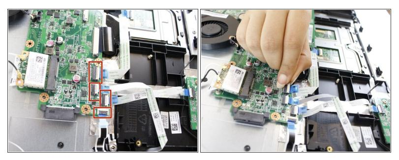
• Use a spudger to flip up the retaining flaps on the ribbon cable <u>ZIF</u> sockets.
