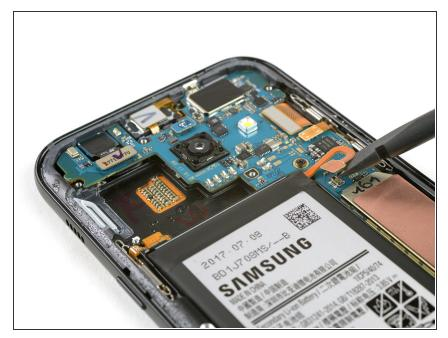
Use the flat end of a spudger to disconnect the battery flex connector.
