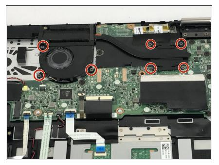
Remove the seven 0.7mm Phillips #00 screws securing the fan in place.
