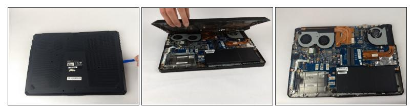
• Use a plastic opening tool to take off the back plastic panel.
