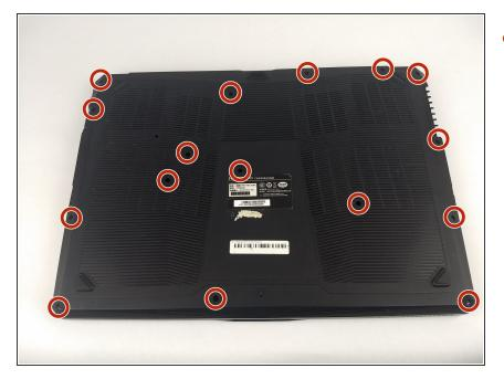
Use a #0 Phillips head screwdriver and unscrew the sixteen 7mm screws on the back of the device.
