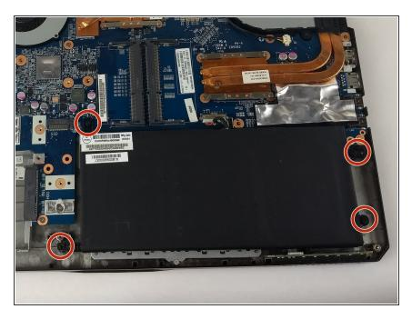
Use a Phillips #0 head screwdriver to remove the four 7mm screws that hold the battery in place.
