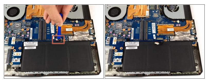
Gently pry off the connecting wires with the plastic opening tool.
