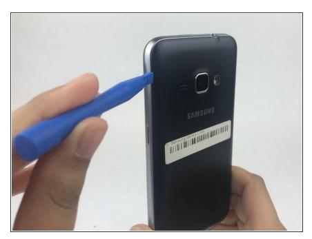
Using a plastic opening tool, pry the divot to the left of the camera to take off the rear case.
