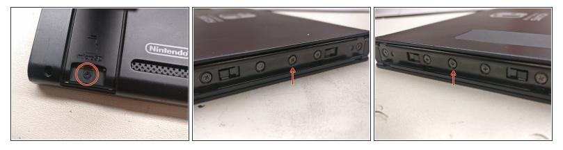
Be sure to lift up the kickstand and remove this sneaky little screw around the SD card slot, and then the center screws on both sides of the device, where the Joycon brackets are screwed in place.
