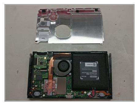
You can now gently pull the metal plate off and set it aside, revealing the tightly designed internals of the switch, along with your battery.
