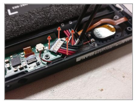
• To remove the battery, take some tweezers or a spudger and carefully pop the connector off vertically; it looks like it might come out perpendicular to the board, but it comes straight off with some gentle prying from underneath.
