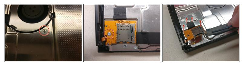
• Take out the center screw, near the blower fan, and the screw in the small SD card reader assembly. Then using tweezers or a spudger, carefully remove the SD card reader and detach the flex cable from the board; you can do this by carefully sliding a spudger under the area covered by the foam and gently prying up. it comes off fairly easily.
