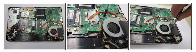
Remove the two 5mm screws on the fan assembly using a Phillips #0 screwdriver.
