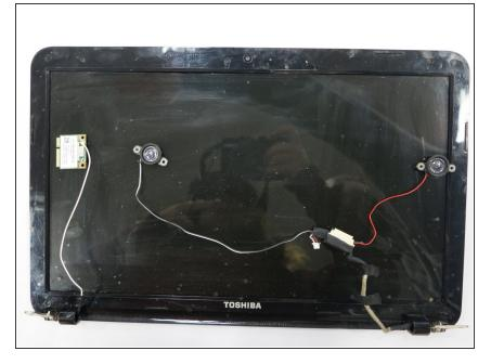
The removed laptop screen should have the daughterboard and speakers attached to it via wires upon removal.
