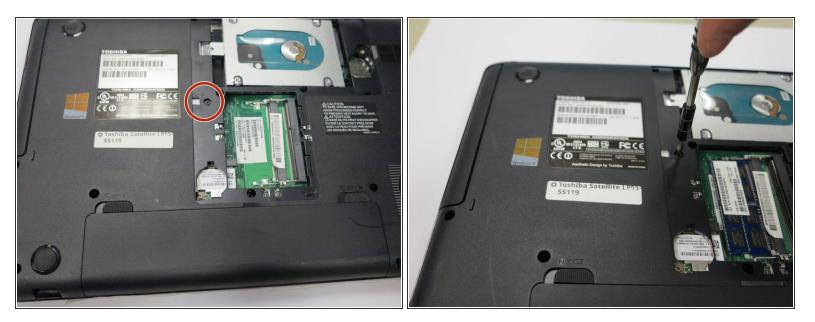
• Using a Phillips #0 screwdriver, remove the single 3mm screw.
