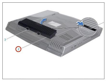
Push the NEW battery pack into the battery bay until the battery pack clicks into place.
