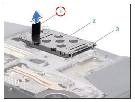
• Using the pull-tab, lift the hard-drive assembly out of the hard-drive bay.
