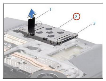
• Place the hard-drive assembly in the hard-drive bay.
