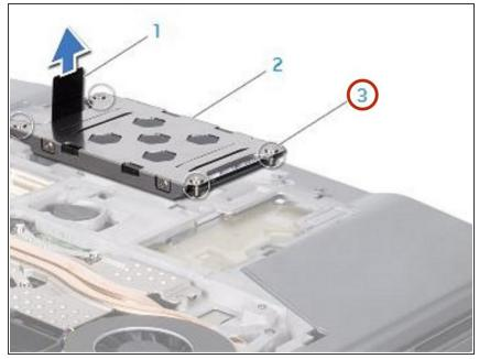
Align and tighten the four captive screws that secure the hard-drive assembly to the hard-drive bay.
