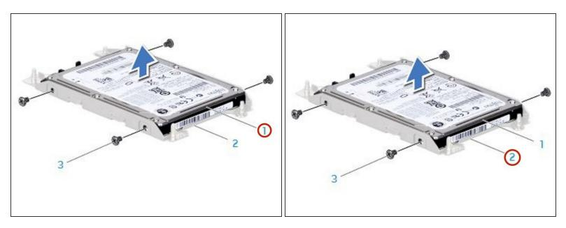
• Place the hard drive in the hard-drive bracket.
