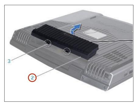
• After the Battery Pack pops up, remove the Battery Pack.
