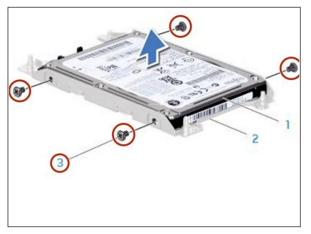
Replace the four screws that secure the hard drive to the hard-drive bracket.
