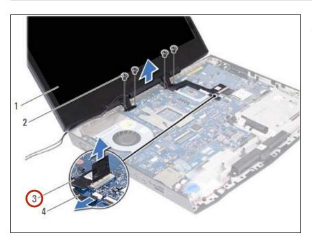
Connect the display cable and the logo-board cable to the connectors on the system board.
