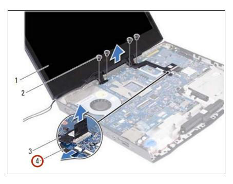
Disconnect the logo-board cable from the connector on the system board.
